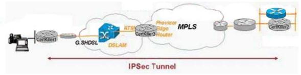
With an IPSec tunnel established between remote Router A and head-end router B, how can the Service Provider Edge Router identify Voice over IP packets flowing through the IPSec tunnel from a Cisco 7960 IP phone?
