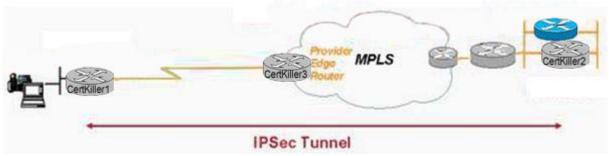
With an IPSec tunnel established between remote Router A and head-end router B, with Compressed Real-Time Protocol (cRTP) configured on the serial interface of Router A, what impact will the cRTP configuration have on the Voice over IP packets flowing through the IPSec tunnel from a Cisco 7960 IP phone?
