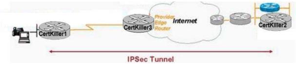
Assume Router Certkiller 1 is configured for split tunneling. If the Internet Service provider was asked by the customer to provide a guarantee of at least 60 percent of the WAN link between Router Certkiller 1 and Router Certkiller 3 for encrypted traffic, what would be the best means of identifying this traffic to their QoS Service Policy?
